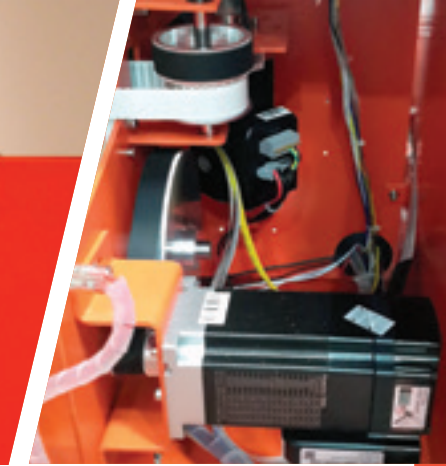
X and Y integrated motors
