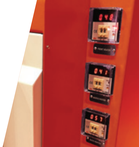
Pre, middle and post-heater controllers
